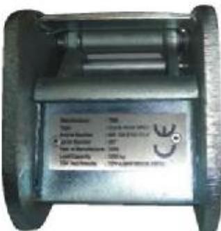
The admissible load of a VINC'I crane hook is 15 kN. Operating the crane hook is quite simple, open the spring loaded safety lever as far as possible. Then position the crane hook on to the panel profile until the cross bar engages completely in the profile groove, let the safety lever back in order to lock the crane hook while lifting large size panel units, take care that each crane hook is attached so that the crane hook touches an inner side profile avoiding any slipping.
