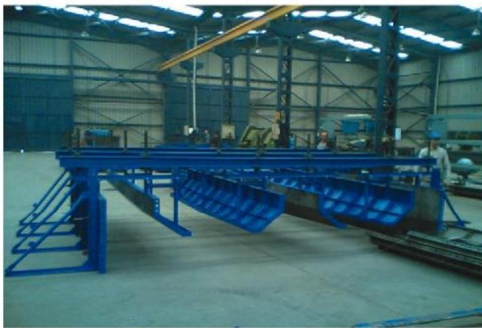
Invert formwork being pre-checked at TMS workshop
