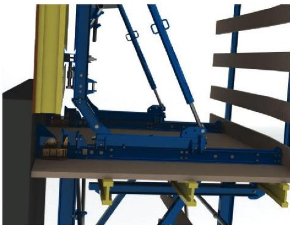
Gear driven Mechanical Formwork carrier
