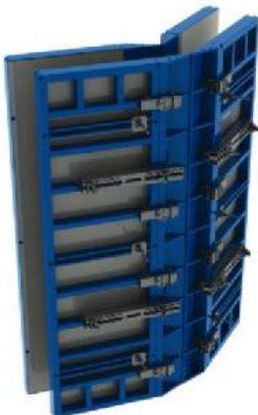
Angled corners are formed by using hinged inside and outside corners. Walers should be applied to the outside corner assembly in order to provide accurate alignment and correct load distribution. When timber fillers are used for compensation, panel connection should be done by CONTI locks. Adjustment range: 75° to 180°
