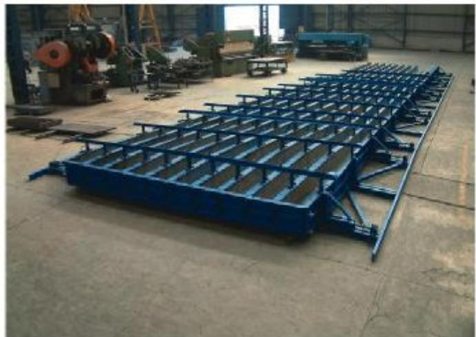
Precast peripheral wall formwork for self compacting concrete.
