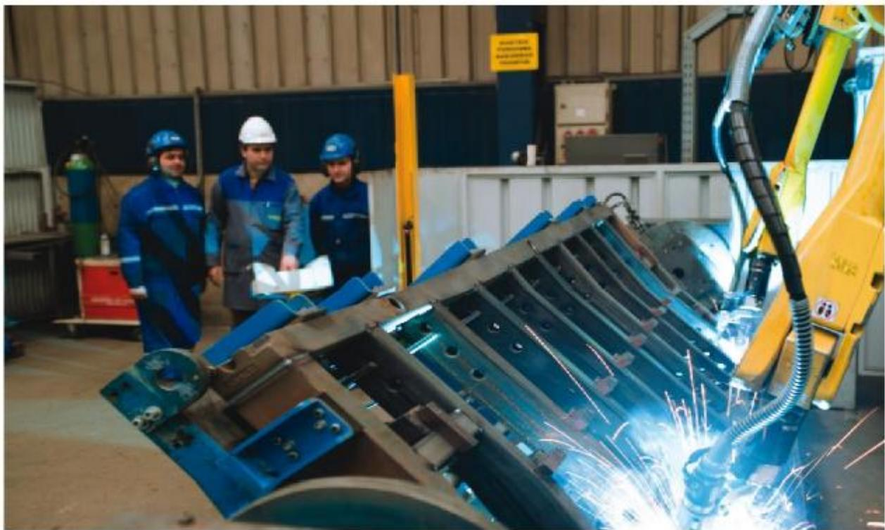
Fully Automated Fixtures and Robotic Welding has been applied for VINC'I production.
